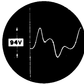
AFC OUTPUT V1013 PIN 5 Y-ATTENUATION 100:1
